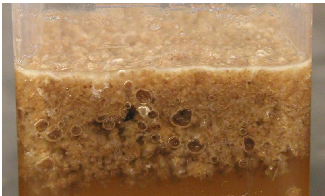
Figure 2. Simultaneous saccharification and fermentation (SSF) of corn stover with P. chrysosporium and E. coli K011 (day 3), clearly showing the formation of carbon dioxide gas bubbles.
