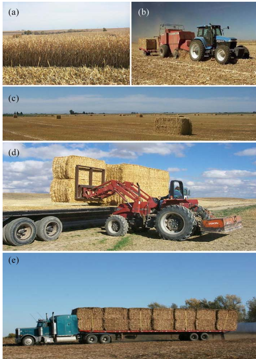
Figure 22. (a) Corn stover a typical corn field, (b) Harvesting and baling of corn stovers, (c) A corn stover bale in the square format, (d) The loading of bales onto a flat-bed semi-tractor trailer, (e) Loaded bales being transport (Hess et al. 2009).
